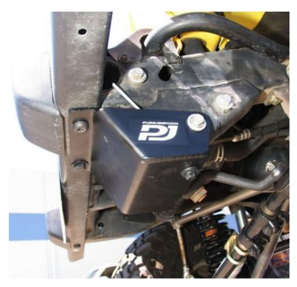
1 - Skidplate 2 - 1/2" x 1" Bolts 1 - 1/2" Lock Nut 3- 7/16" Flat Washer 1 - 5/16" x 1 Self Tap 1 - 5/16" Flat Washer
